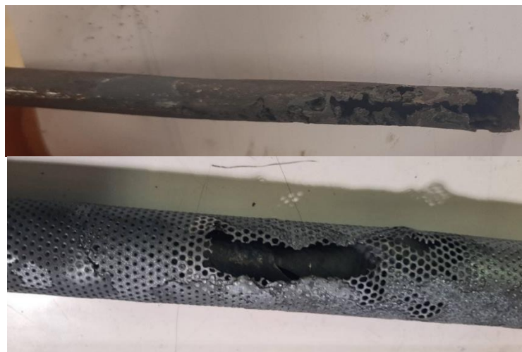
Figure 12 - Location of the burner fracture as a result of the high-temperature oxidation
