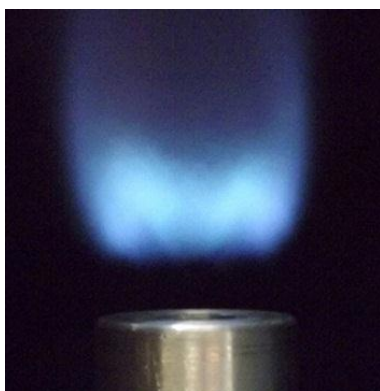
Figure 9- Lifted flame in M-Shape condition
