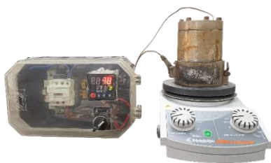
Figure 2- Stainless-steel reactor equipped with temperature control for the esterification reaction
