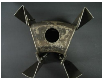
Figure 10- Combustor sector and test section holders
