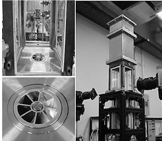
Figure 1- Images of the experimental swirl-stabilized combustor[8] used in this study
