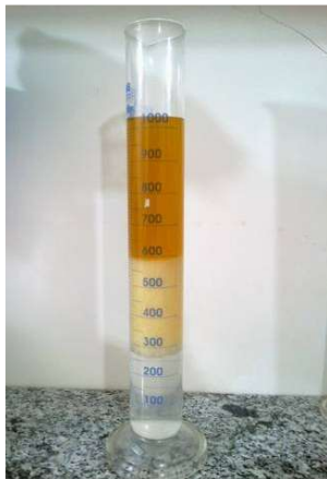
Figure 2- The first stage of water washing and formation of three phases of fuel, soap, and oil شکل ۲- مرحله اول آب‌شویی و تشکیل سه فاز سوخت، صابون و روغن
