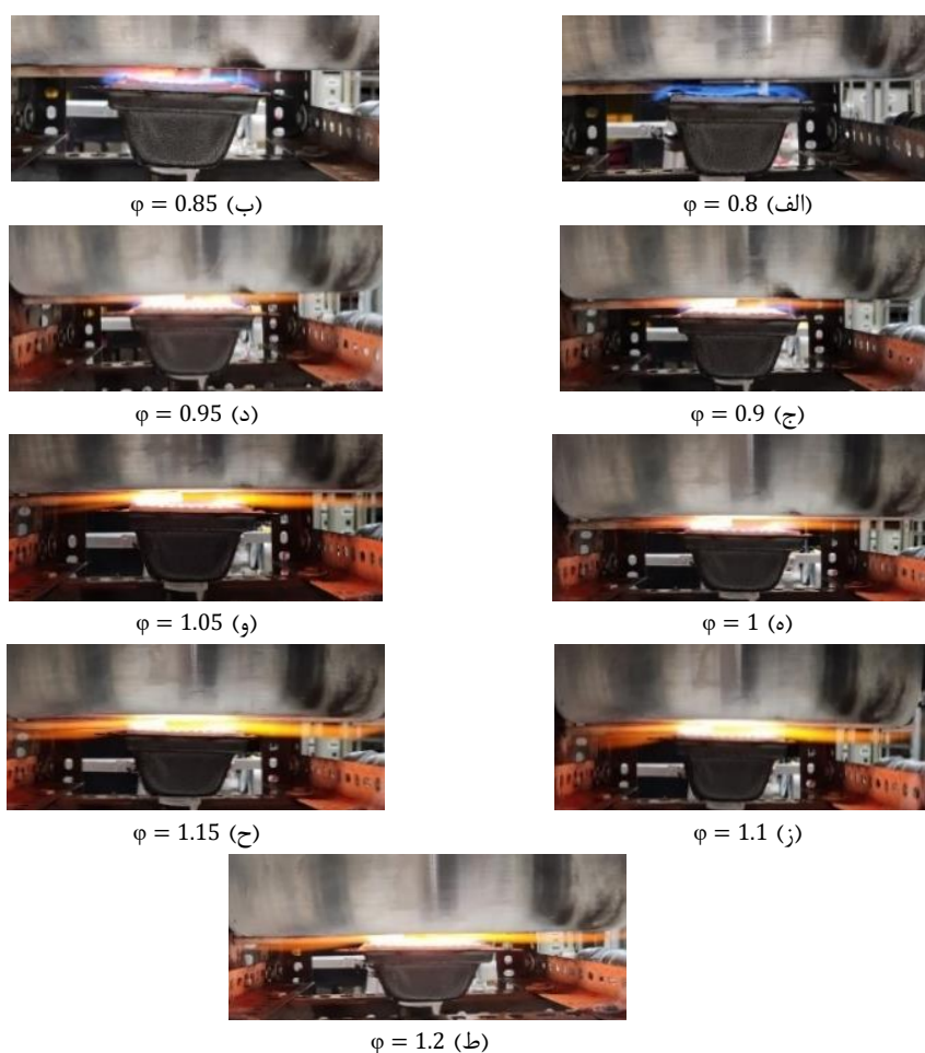
Figure 7- Change in shape and flame regime from equivalence ratio 0.8 to 1.2 in thermal power kW 9.83
