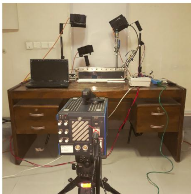
(a) Figure 1- A) Schematic view of the laboratory system: 1. Ignition system including spark plug, 2. Pressure sensor, 3. Gas inlet and outlet, 4. Gas injection, 5. High speed PCO camera, 6. Perforated plates or porous barriers and B) Real view of laboratory system
