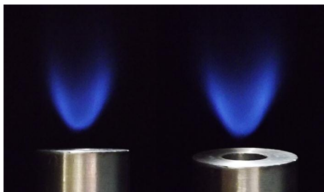
Figure 8- Lifted stable flame of swirler-1
