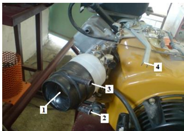
Figure 7- Mixture Chamber and Engine connections (1- Air inlet, 2- CNG inlet, 3- HHO inlet, 4- Engine air intake valve lever)
